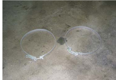
2 x clamps to clip filling trunks of the ElcoRock bags to funnels.
